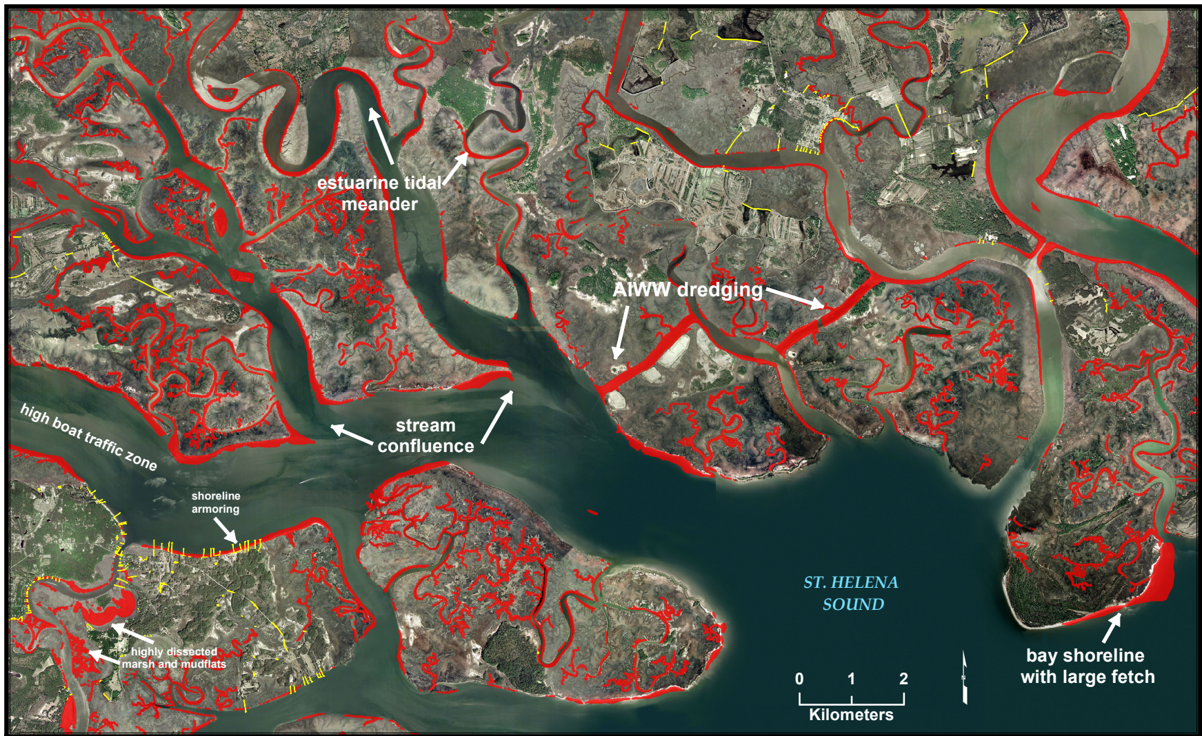
Figure 4-2. Map depicting erosion (red) with shoreline structures (yellow) and factors potentially influencing erosion patterns at specific areas.
