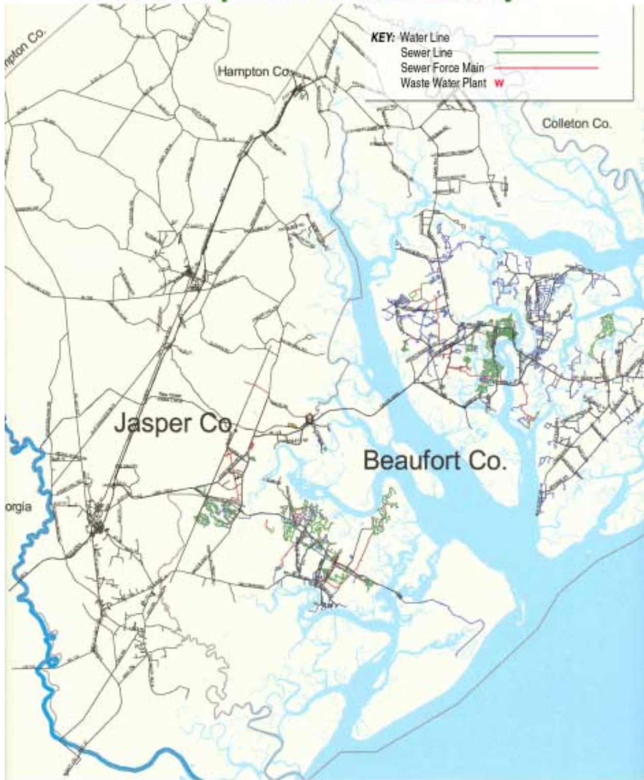
Figure 2.1 BJSWA Water and Sewer lines
